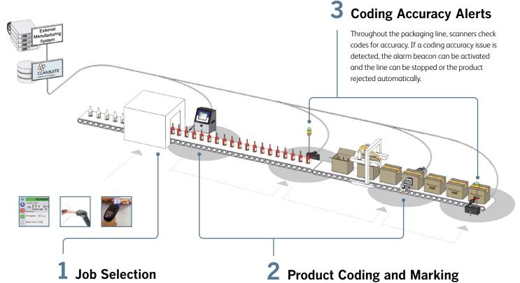
The product or appropriate code can be selected at the CLARiSUITE<sup>™</sup>-installed PC or Videojet printer. Or, a bar code can be scanned from a work order or from the product itself with a hand-scanner.
